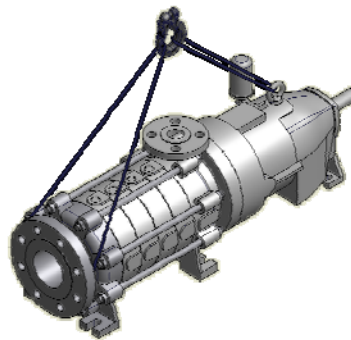
Fig. 5: lifting the pump
