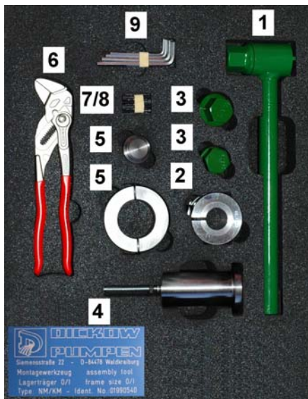
Fig. 10: Special tools frame 0 / I
