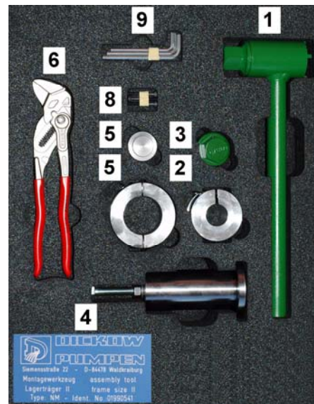
Fig. 11: Special tools frame II
