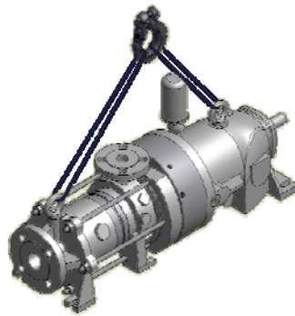
Fig. 5: lifting the pump
